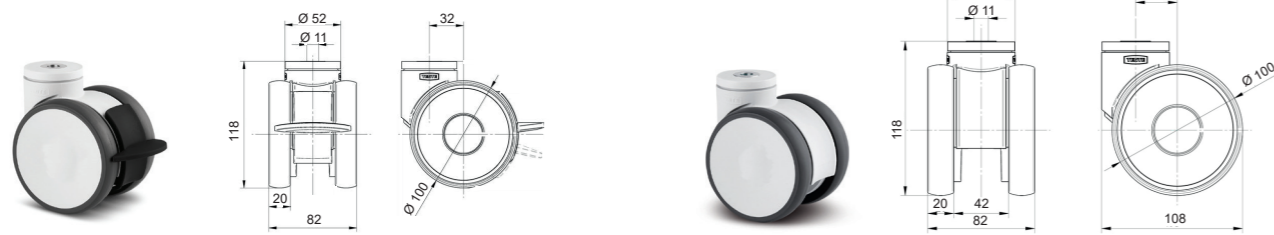
PZ1540 Swivel castor with total lock and bolt hole (Code 01)
