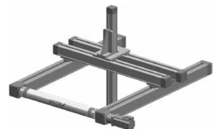
WDS - coupling for multi-axis linear module
