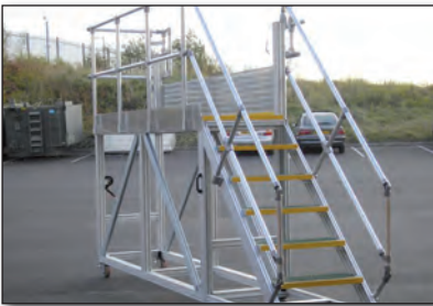
Flask inspection platform
